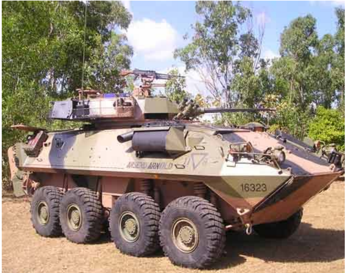
The ASLAV 25, an amphibious eight-wheeled armoured vehicle currently on patrol in Al Muthanna Province in IRAQ, currently in service with 5/7RAR (Mech).
