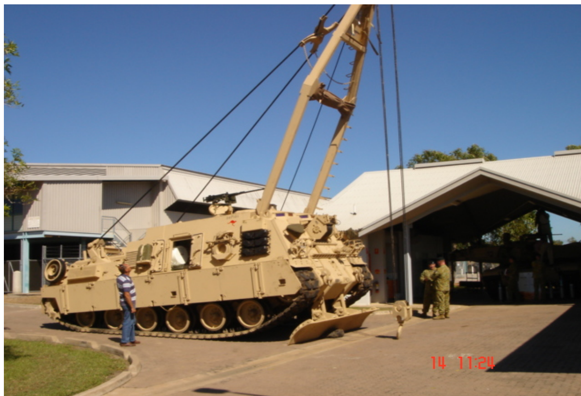
Above and Below : Hercules, the Armoured Recovery Vehicle.
